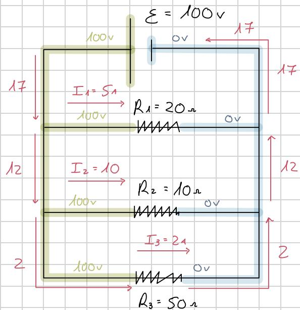
$$I_1 = \frac{V_1}{R_1} = \frac{100}{20} = 5$$
