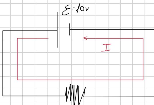
$$\left. \begin{array}{l} R_1 = 5 \Omega \\ V = 10V \end{array} \right\} I = \frac{V}{R} = \frac{10}{5} = 2A$$
