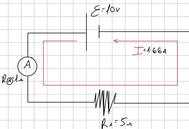
$$I = \frac{E}{R_1 + R_2} = \frac{10}{5+1} = \frac{10}{6} = 1.666\overline{6}$$
